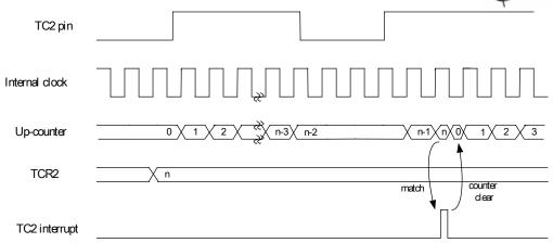
Fig. 22. Window Mode Timing Chart
